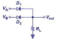
7.3 ( b ) What is the diode model of the following figure ? (a) Constant voltage model (b) Exponential model (c) Ideal model (5%)
