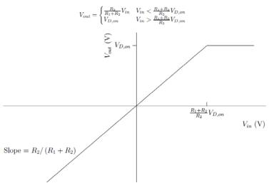
6. (10%) Using the constant voltage mode, plot the input/output characteristic of the following circuit.
