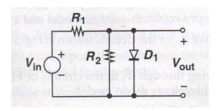
6. (10%) Using the constant voltage mode, plot the input/output characteristic of the following circuit.
